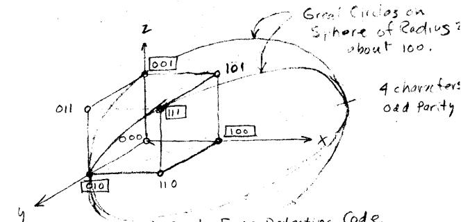
Fig. 2,4 a Example of Single Error Detecting Code Minimum Distance D(x,7) = 2
